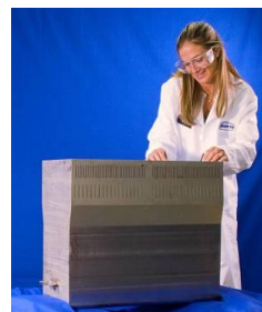
1/4 scale SMR reactor Device: 22" x 12" x 24" Capacity if operated: 0.33 million ft 3 /day of H 2
