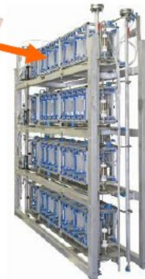
Corning® Advanced-Flow™ Glass Reactor
